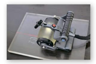
The Phased Array Wheel Probe is newly released by SIUI, especially good for fast testing of composite plates and pipe corrosion.
