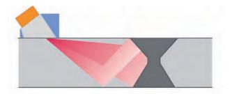
For one phased array probe, multi groups of element and multi angles can be applied for scanning at the same time, fully covering the welding area and enhancing the inspection efficiency.
