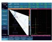
This is to help set a gate over an area and adjust the gain for this area regardless of the global gain. It is very useful for inspection of forgings and castings with allowing independent gain control of the area under the gate with the BEA for backwall echo monitoring.
