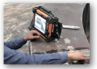
Suitable for flat butt welds inspection.
