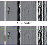
TOFD measurement is easy and useful. The flaw height and length can be measured by moving the reference line. The measurement result is clearly shown in the data table.
